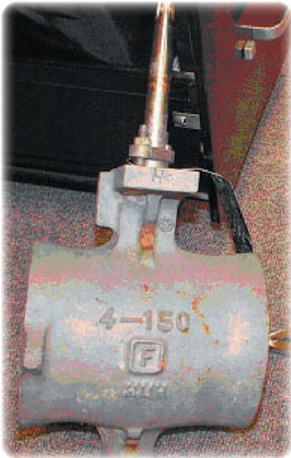
Outside view of a typical valve used to control pulp in a paper mill.
